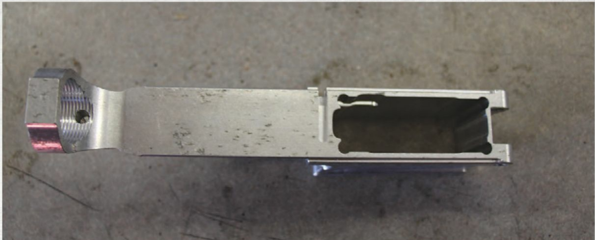
EPL with trigger group cavity yet to be machined in.
