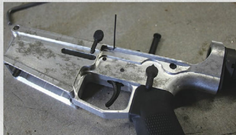
Above: Bolt release is held in a bit differently than .223 AR: pin is held in by a tiny screw. This allows operator to adjust tension.
