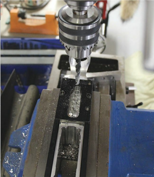
Above: First part of cavity finished, with jig for shelf in place. Depth for shelf is .525 inch.
