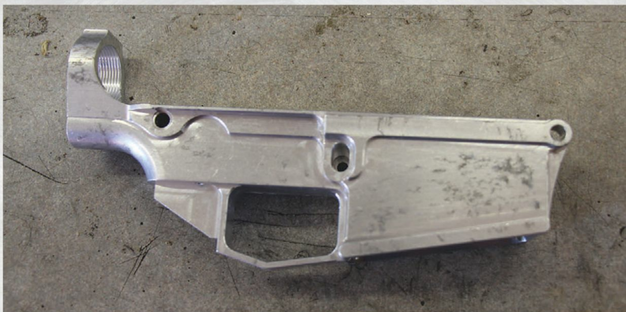
Side view shows no dents where trigger pins should go.
