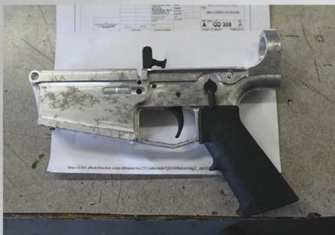
Trigger group installed, lower is ready for engraving and finish.
