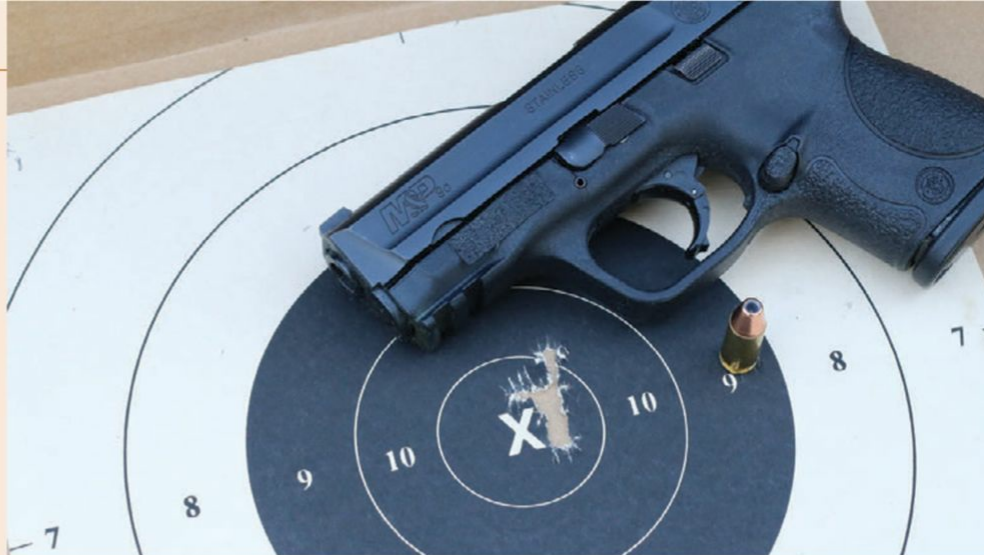
Hornady 115-grain HAPs over 4.4 grains of Bullseye alongside 25-yard timed-fire target. Load shot well out of a variety of service handguns.
