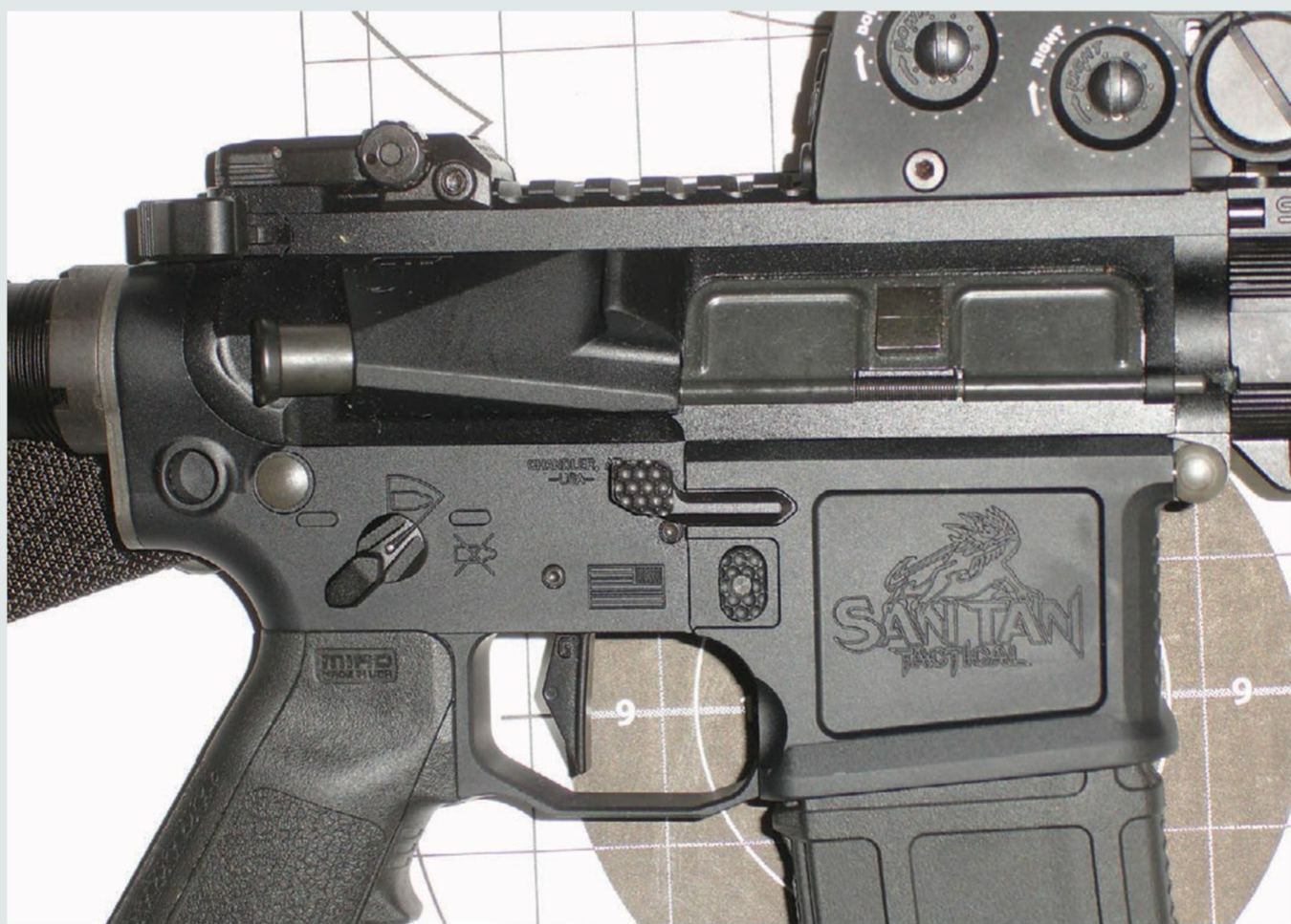
San Tan Tactical lower receiver shows Talon 45/90 ambidextrous safety that changes a 90-degree throw to a shorter 45-degree throw.
