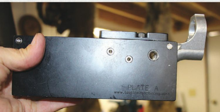
Below: Trigger pin holes are in and lower is ready to machine out the cavity. Even without further machining, it is now considered a firearm by the ATF.
