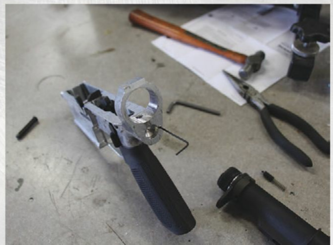
Below: Rear takedown pin detent is held in by a tiny screw instead of the stock plate, and is adjustable for tension.
