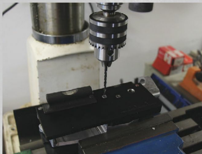
Above: Set up in the press for trigger pin holes and selector. Make sure workpiece is level so holes go through straight.
