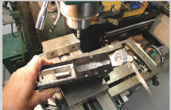
Above: First part of cavity finished, with jig for shelf in place. Depth for shelf is .525 inch.
