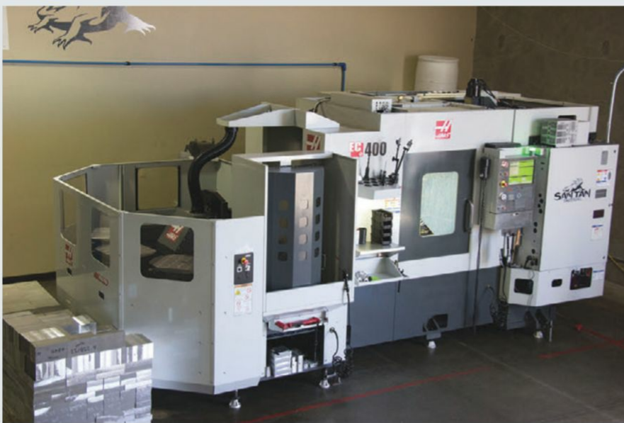
San Tan Tactical machines STT-15 directly from a billet of 7075-T651 aerospace-grade American aluminum on state-of-the-art Haas CNC machinery. Photo: San Tan Tactical
