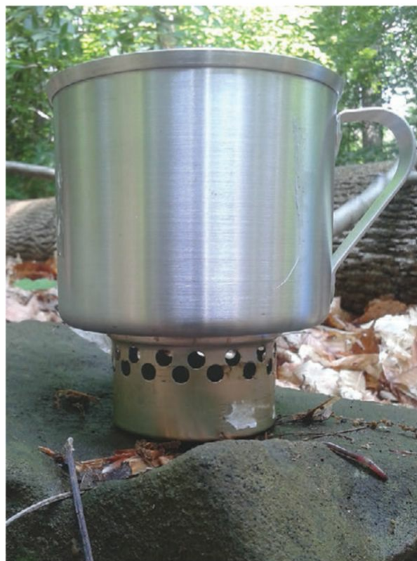
Super Cat alcohol stove is lightest weight stove author has ever heard of. It is made of a cat food can with holes punched around its rim.
